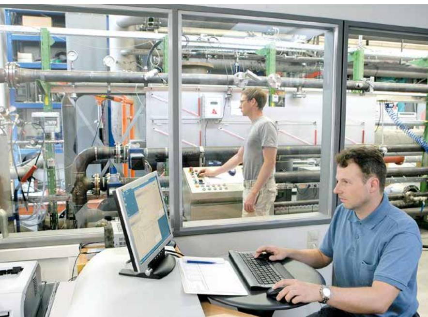
In order to guarantee the precision of the measurement and control systems, the pressure, temperature and loading conditions which will later occur in the customer's plant are simulated exactly using the appropriate gas mixture.
